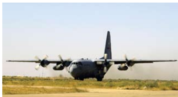
Figure 13-7. The C-130 Hercules. The C-130 is the most versatile fixed-wing aircraft used for aeromedical evacuation. It can carry up to 70 litters and can operate in austere locations. Reproduced from: US Air Force Link photo library. www.af.mil/shared/media/photodb/photos/031030-F-9629J-005.jpg .
