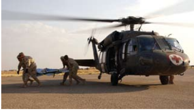
Figure 13-1. The UH-60 Black Hawk. The UH-60 Black Hawk can hold up to six litters for patient transport and is the Army’s front-line helicopter for aeromedical evacuation in Iraq and Afghanistan.
