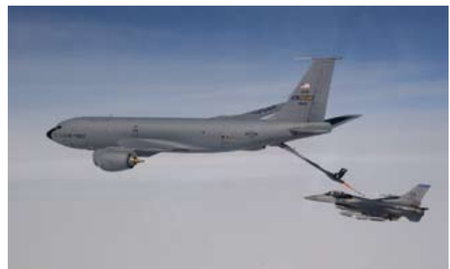
Figure 13-4. The KC-135 Stratotanker. The KC-135 is used primarily for air refueling, but it can be configured with patient-support pallets and used for aeromedical evacuation.
