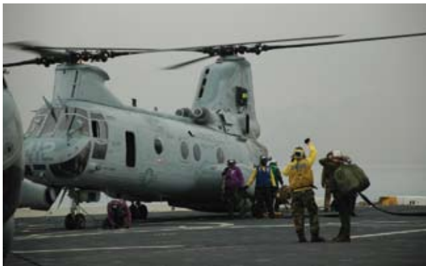
Figure 13-2. The CH-46 Sea Knight. The CH-46 can accommodate up to 15 patients and was used extensively by the Marines during the battle of Fallujah in November 2004. Here, Marine Reserves—the “Moonlighters” from Marine Medium Lift Helicopter Squadron 764, based at Edwards Air Force Base, Calif—pause for refueling and servicing by the US Navy flight deck crew aboard the USS New Orleans , participating in a nine-country training exercise called Partnership of the Americas, July 3, 2010. Photographer: MSgt Peter C Walz.
