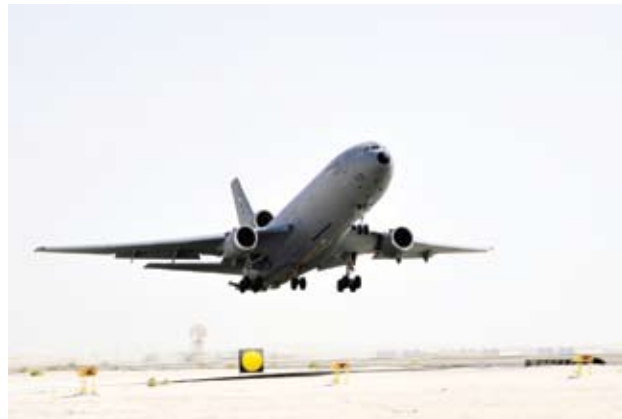
Figure 13-6. KC-10A Extender. The KC-10A is another air refueler that can be configured for aeromedical evacuation when loaded with patient-support pallets. Reproduced from: US Air Force Link photo library. www.af.mil/shared/media/photodb/photos/091013-F-3140L-112.jpg .
